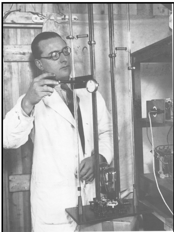
George Brown G5BJ works on a VHF Lecher Line transmitter (G6SL) in the roof-top laboratory at Stratton's Balmoral Works, 1935. Signals were received in New York.
